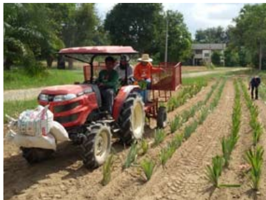
Figure 7 Pineapple transplanter attached with tractor 39 Hp Testing performance at farmer field, Khon Kaen Province
