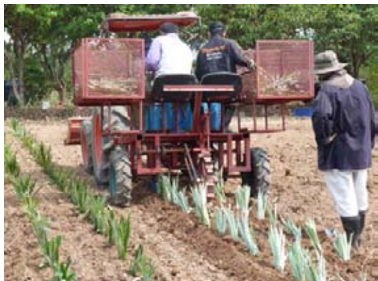
Figure 6 Pineapple transplanter attached with tractor 45 Hp, testing performance at Nong Khai Research and Development Center Nong khai Province
