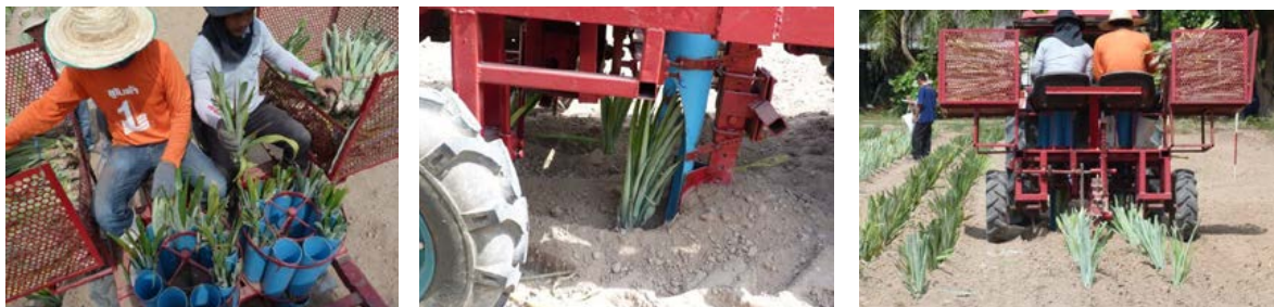
Figure 5 (a) Entering suckers planting pineapples with 2 labors (b) Characteristics and drown out pineapples suckers through the tube (c) Pineapple Cultivation double rows in a row spacing of about 1 meter
