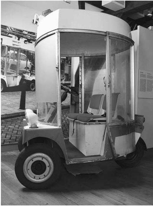
FIGURE 5.1 A Dutch Witkar (White Car) from the 1970s. The all-electric vehicles featured a 24-volt motor, three wheels, two seats, and a maximum speed of 30 km/h (about 18 mph).
